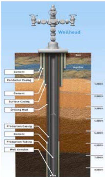
Figure 1. Standard casing diagram for an oil and gas well.
