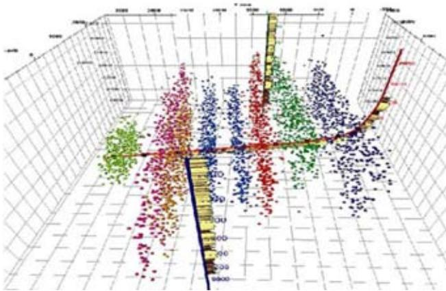
Figure 3. Example of a microseismic HF mapping
